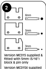
with 3mm (1/8"), 5mm (3/16") & 6mm (1/4") blocks & pins with 5mm block & pin factory fitted.
