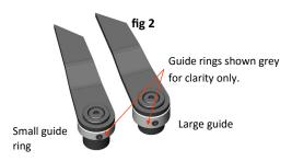
**4b** When rolling round or square bar up to 8mm place the steel between the two guide rings.
