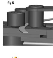
When rolling or bending materials less than 5mm thickness, it is advisable to use the Side Roller Sleeves "B" provided. This reduces clearance to produce better angle bends and roll smaller radii.
