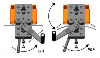
Screw stop "A" can be used to maintain the applied pressure, thereby allowing both hands to be used for operating the winding handle. By repeating this it is possible to produce an infinite variety of curves and circles.
