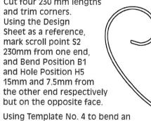
angle of 100 degrees at B1 and repeat with the other 3 connectors. Next punch holes H5 in all four and then form scroll to \$2 again in all four making sure the scrolls are as identical as possible.
