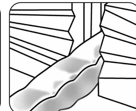
Applying gentle curved indents down the length of the tube achieves a decorative hammered effect.
