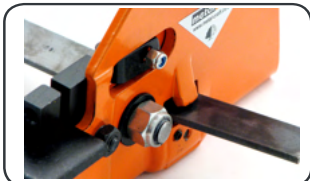
Cuts steel bars.
